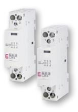
Important: At an ambient temperature of  $t \le +40$  °C, the maximum number of contactors that can be installed side by side is 3 units. At temperatures from +40 to +55 °C, the maximum is 2 units. When using more units, it is necessary to install an intermediate spacer IKV, Code No. 002464074.
